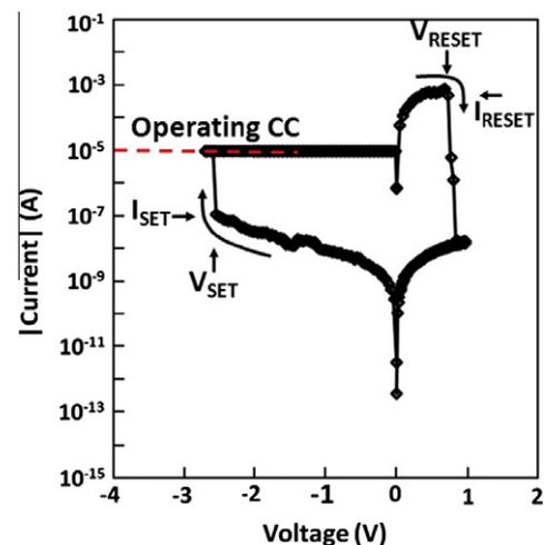
Fig. 2. Plot of log |current| vs. top electrode voltage showing a typical complete bipolar switching cycle for a  $10\ \mu\text{m}$  by  $10\ \mu\text{m}$  device with a gradual form CC of  $500\ \text{nA}$ .
