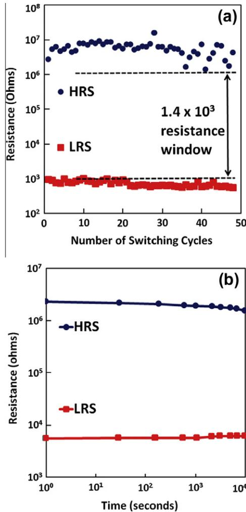
Fig. 3.  $R_{HRS}$  and  $R_{LRS}$  vs. (a) the number of switching cycles for the device from Fig. 1(b) and (b) vs. time for a similar device.
