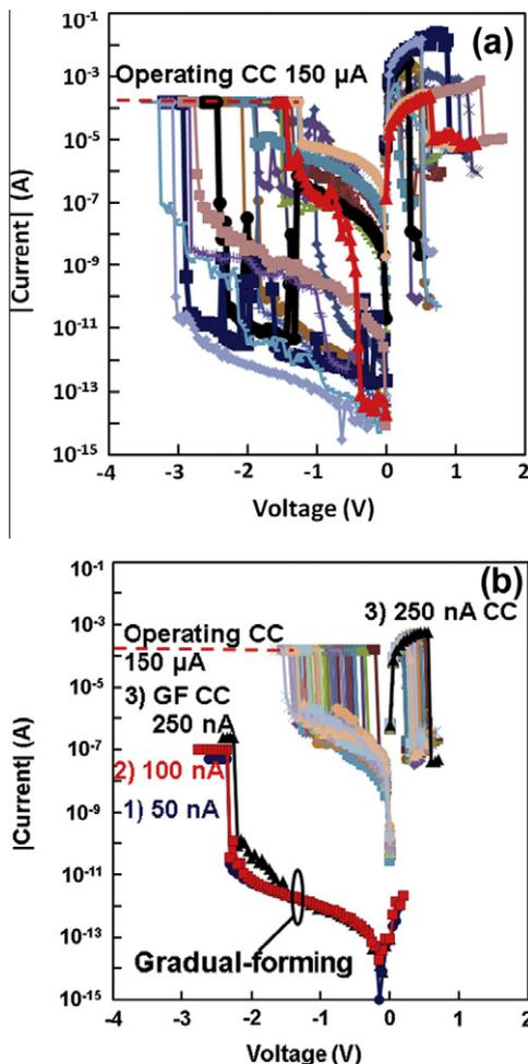
Fig. 1. Plot of log |current| vs. top electrode voltage for a  $50\ \mu\text{m} \times 50\ \mu\text{m}$  device with an operating CC of  $150\ \mu\text{A}$  (a) without the GF process and (b) with a GF CC of  $250\ \text{nA}$ .
