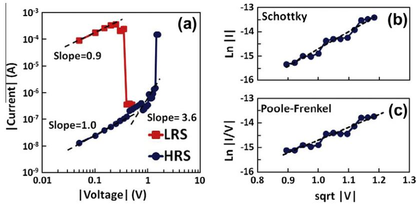
**Fig. 5.** (a) Plot of log |current| vs. log |voltage| for 50  $\mu\text{m} \times 50 \mu\text{m}$  using a 150  $\mu\text{A}$  operating-CC along with (b) Schottky plot of  $\ln |I|$  vs.  $\sqrt{|V|}$ , and (c) a Poole–Frenkel plot of  $\ln |I|/|V|$  vs.  $\sqrt{|V|}$  for the high slope part of the HRS data.
