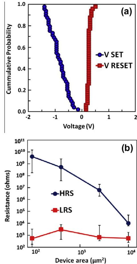
Fig. 4. (a) Cumulative probability plot of  $V_{SET}$  and  $V_{RESET}$  for a 50  $\mu$ m  $\times$  50  $\mu$ m device with gradual forming and an operating-CC of 150  $\mu$ A. (b) Plot of the median HRS and LRS vs. device area (error bars indicate minimum and maximum values).
